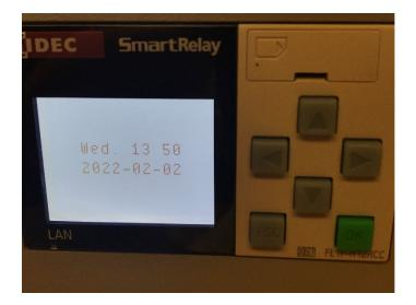
The above image demonstrates what the PLC display will show when the unit it initially turned on.
