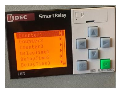
The factory settings for all of the Counter features will be set at 3 cycles (as measured by the proximity switch).
