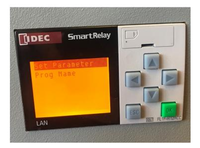
Choose the Set Parameter option by highlighting and clicking OK. The next screen (shown below) will display Counter 1-3, Delay Time 1-3, and Spray Time 1-3.
